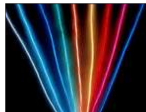
Several colors of EL Wire. glows when electricity runs through it.
